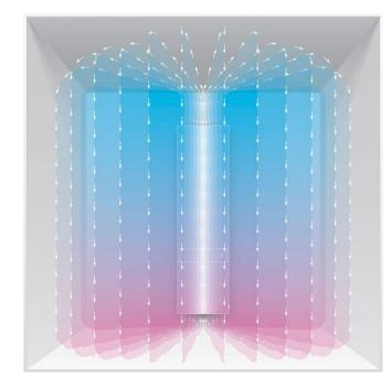
Thanks to its narrow, tower-like design, the UV-C FiltAir provides ideal airflow, thus moving and cleaning the entire air in the room. Properly selected UV-C FiltAir air sterilizer cleans the indoor air five times an hour.
